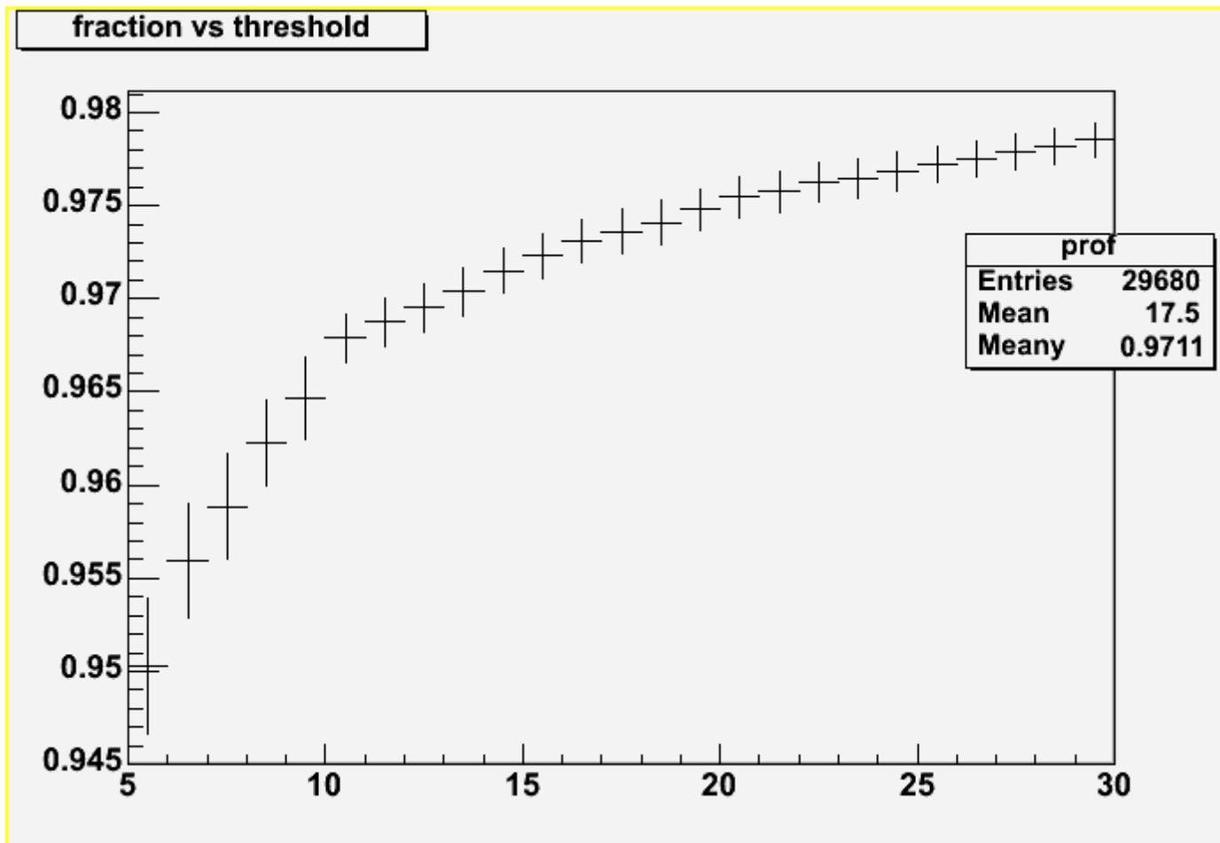
Distribution of energy in TileHitVector: fraction of energy that releases in time interval from 0 to threshold time in ns, e.g. 0.965 at 10 ns point means that 96.5% energy deposited in first 10 ns
