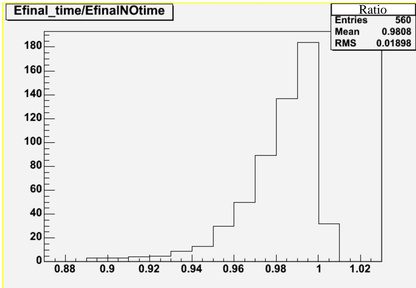
Ratio of energy after FitFilter with time saving to energy after FitFilter with time equal to zero.
