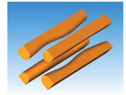
Figure 2.1a. Electrodes of accelerating structure with spatially-homogeneous quadrupole focusing (RFQ)
